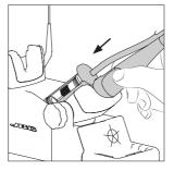
When the tool is returned to the stand, the temperature falls to the preset Sleep temperature.
