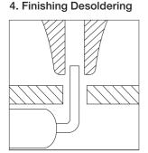
After releasing the tool button there is a slight delay until the vacuum pump of the desoldering module stops. This makes sure that the tip duct is completely empty.
