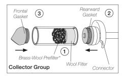
Afterwards, insert the frontal gasket into the other side of the glass solder-collector (3).
