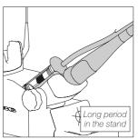
After longer periods of inactivity, the tool goes into Hibernation Mode: the power is cut off and the tool gradually cools down to room temperature.
