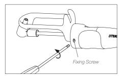
Loosen the fixing screw.
