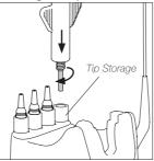
To remove the tip from the spanner, simply place the tip in one of the holes of the tip storage, screw it in lightly (only approx. 1 turn) and pull the spanner out.
