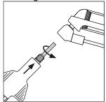
Grab the new tip with the spanner. Fit it into the heating element and screw it in with the spanner. Screw the tip all the way in so that the union is air-tight. **Note:** Do not screw the tip in too tightly.
