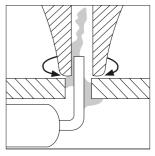
Press the tool button long enough to suction the liquefied solder.
