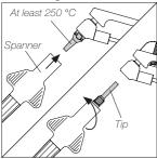
Use JBC's spanner to unscrew the tip. The tip will remain attached to the spanner so that it can be moved safely.
