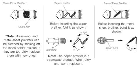
Assembly Sequence using brass-wool prefilter:
