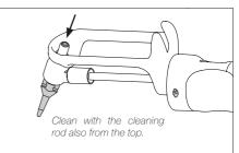
Remove the solder collector group, leave the tool on the stand and clean the tip with the cleaning rod also from its top.
