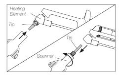
If the heating element has a tip on, remove it with the provided spanner.
