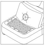
A damp sponge is the softest cleaning method. When working, keep the sponge damp using distilled water to avoid tip wear.
