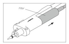
3. Use the cleaning brush (ref. 0008297) to clean the solder collector inside or replace it
