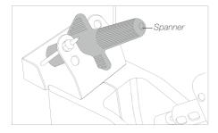
Place the Soldering Iron in the extractor and remove the tip.
