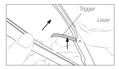
Open DPM by lifting the lever and the trigger.
