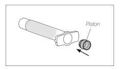
Fit the piston into the barrel previously filled with solder paste.
