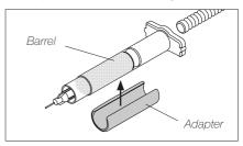
For 3 cc syringes the adaptor is needed. Assemble the adapter by clipping it onto the barrel.
