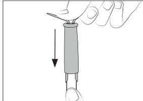
Push the grip with the tabs onto the handle.
