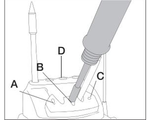
Use the holes to fix the cartridge as follows:
