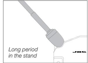
After longer periods of inactivity, the power is cut off and the tool cools down to room temperature.
