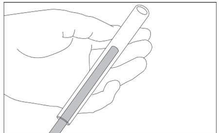
Check the filter and replace it if it is dirty or damaged.
