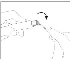
Enter, not deeper than 8mm, a small shaft or screwdriver, lift and pull the sealing plug. Never use a cartridge to do this operation.
