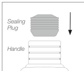
**Note:** The chamfered side has to be positioned towards the handle.
