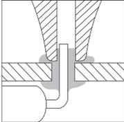
When the solder melts, gently move the tip in a circular motion.
