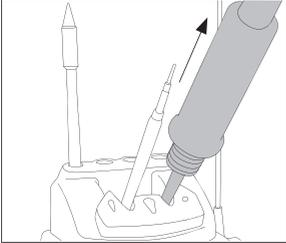
Place the cartridge in the extractor and pull the handle to remove it.
