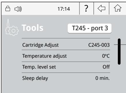
Insert the cartridge model and the station will recognize its characteristics (size and shape) to provide better temperature precision.
