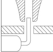
Remove the tip while maintaining the suction to make sure all the solder is removed from the joint.
