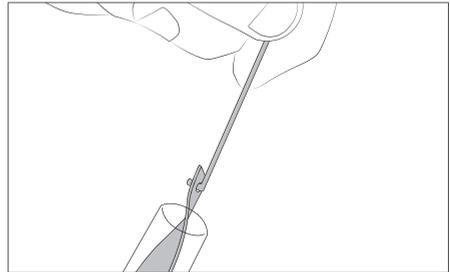
Remove the coil and clean the inside of the glass solder collector with the cleaning stick.
