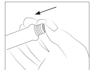
Push the sealing plug inside the handle until the sealing plug and handle edges are aligned.
