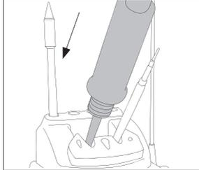
Place the handle on top of the new cartridge and press down.
