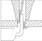
Press and hold the tool button to start the suction and continue the movement completing 3 or 4 circles.
