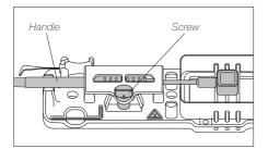
**3.** Once in place, lock the screw and connect the handle to the stand.
