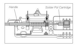
**2.** Place the handle with its solder pot cartridge previously inserted. Be careful to position it correctly.
