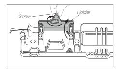
1. Unlock the screw and open the holder.
