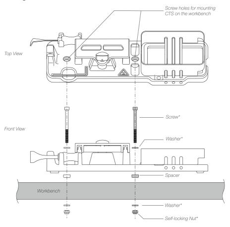
To protect the stand's rubber feets from wear and tear when fixing CTS in place put the spacers (see packing list) between the stand and the workbench.
