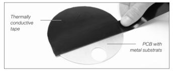
**2.** Place the PCB with the tape on the PCB Holder. After use, it can be easily removed without leaving any residue. It can also be reused.
