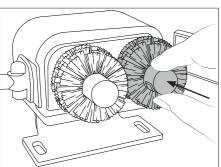
**4.** The Splashguard also works as a tin collector. Clean it and place it back in its position.
