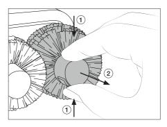
3. Align the brush axis with the motor axis a click is heard. Check if the brushes are
