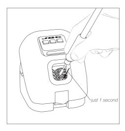
The tip cleaner is automatically switched off if the splashguard is opened during operation.
