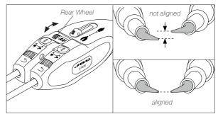
Slightly turn the wheels to align the cartridges as required (1). Then lock the cartridge fixing screws\* (2).
