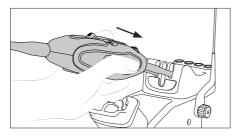
Use the vertical grooves to position the cartridges and place the tweezers onto the cartridges.
