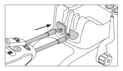
Press the cartridges against the extractor and make sure that the cartridge is inserted up to the mark\*.
