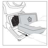
Remove the wiper by pulling it out.
