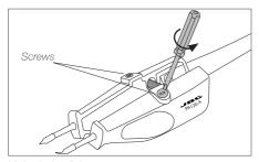
Unlock the fixing screws.
