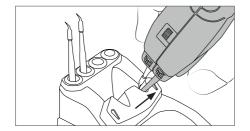
Place the cartridges in the extractor and pull the tweezers to remove them.
