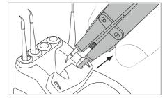
Place the cartridges in the extractor and pull the tweezers to remove them.
