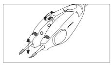
Close the tweezers and the rear wheel allows the cartridges to be equally aligned in a vertical direction.
