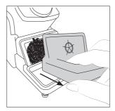
Remove the wiper by pulling it out.
