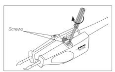
Lock the fixing screws.
