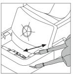
Use the slots to remove the remaining particles.
