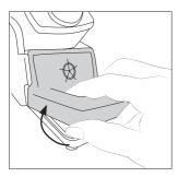
Lift the wiper at its front edge.
