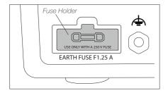
2. Insert the new fuse into the fuse holder and return it to the station.
