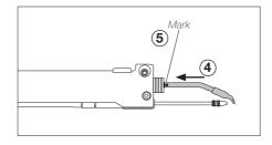
Place a new cartridge into the auto-feed iron (4).
