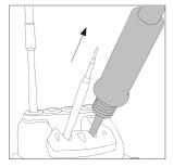
Place the cartridge in the extractor and pull the handle to remove it.
