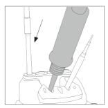
Place the handle on top of the new cartridge and press down.
