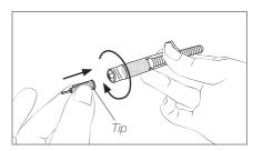
Thread the tip\* onto the syringe barrel.
