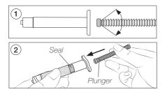
1. Pay attention to the fact that the plunger enters with its cylindrical part in the syringe barrel and the direcction of the teeth angle corresponds to the upper image. Otherwise, the DPM will not work properly.
