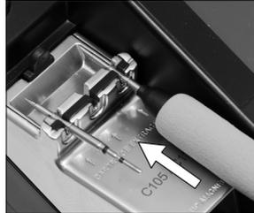
Push the Cartridge into the handle to the ring\*.
