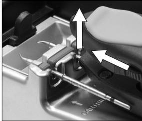
Push the Cartridge into the tool to the ring\*.
