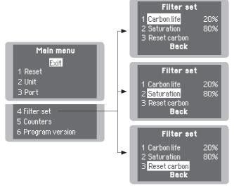
Shows % of remaining life of the carbon filter contained inside the FAE1-200 filter. It is also displayed on the main screen.
