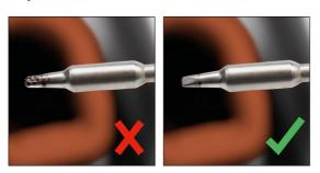
A clean tip is always easier to tin, resulting in higher quality solder joints.
