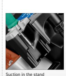
JBC Fume Extractor has an integrated vacuum system that detects when the tool is returned to the stand and automatically absorbs excess of fumes.
