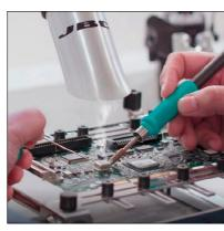
Suction in use Fume Extractor starts up when the tool is lifted from the stand.
