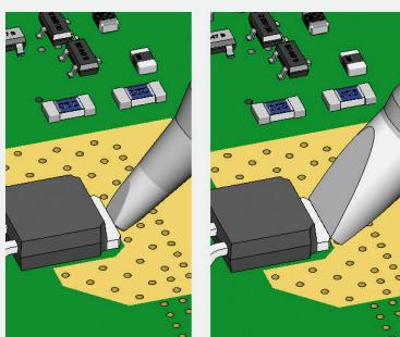
The more mass the tip has, the more heat is accumulated and the **lower is the temperature drop**.
