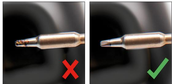
A clean tip is always easier to tin, resulting in **higher quality solder joints**.
