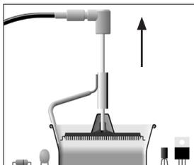
The component lifts off automatically when the solder melts.
