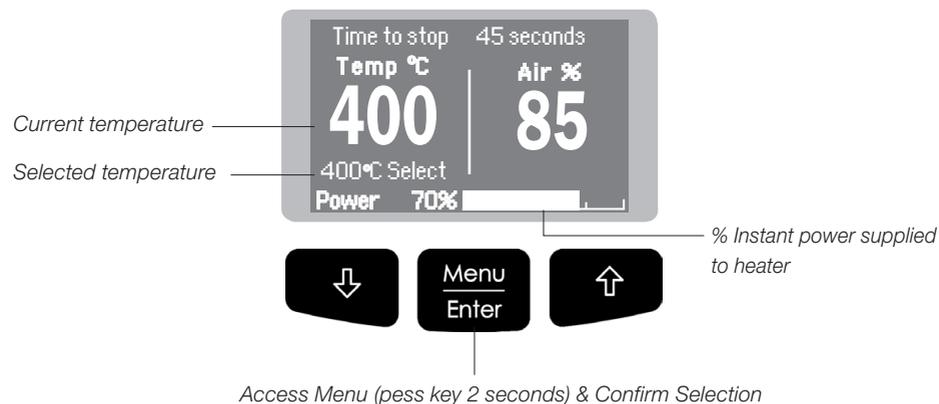
You can switch between operating modes (Manual Mode / Program Mode) by pressing the "increase" and "decrease" keys simultaneously for 2 seconds. (Only when Program mode is ON)
