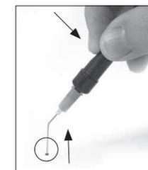
Once the suction is activated, cover the pen hole with your finger and lift off the component.
