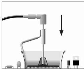
Position the extractor with the appropriate suction cup and press the suction button.
