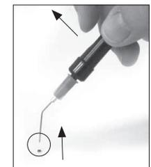
Lift your finger to release the component in the appropriate place.
