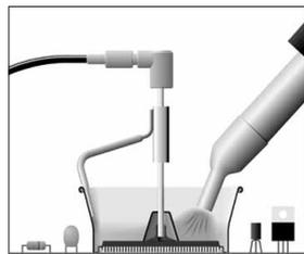
Heat the component by pressing the heater button.
