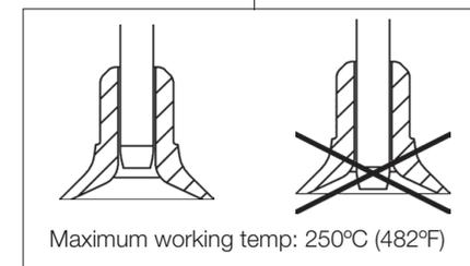
Insert the needle with the appropriate cup for a correct suction process.
