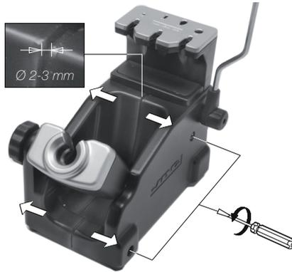
**2.** Remove the screw and place the new S3-B following the same steps conversely.
