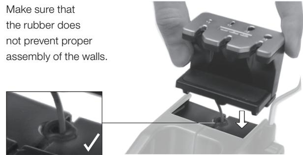
When you place the new S3-B make sure the cable fits snugly and is not pinched for a proper connection.
