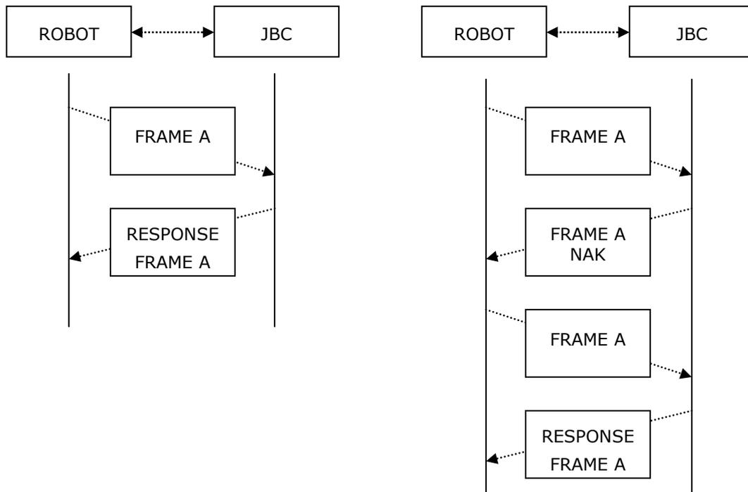
The number of repetitions followed by erroneous frames is determined by the Robot. The JBC equipment does not expect an ACK from the information the Robot sends. If the Robot receives a frame with errors, it cannot ask this to be resent, so that it only can repeat everything once again.
