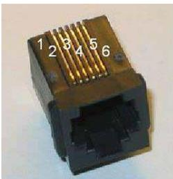
Physically it is type RS-232 with RJ12 connector (RJ-11, only 4 pins are used) and configuration: speed from 1200 to 500000 bps; 8 bits of data; even parity, odd parity or no parity; and 1 or 2 bits of stop (e.g. 19200-8E1). See the following pin distribution:
