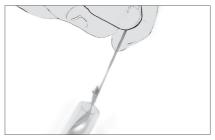
Remove the coil and clean the inside of the glass solder collector with the cleaning stick.
