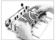
After loosening the SP guide knobs, push the PCB against the SP guide and lift out.
