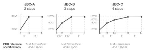
Profiles set using the low position of the PHS-SA Support (28 mm in height between the PCB and the heating area).
