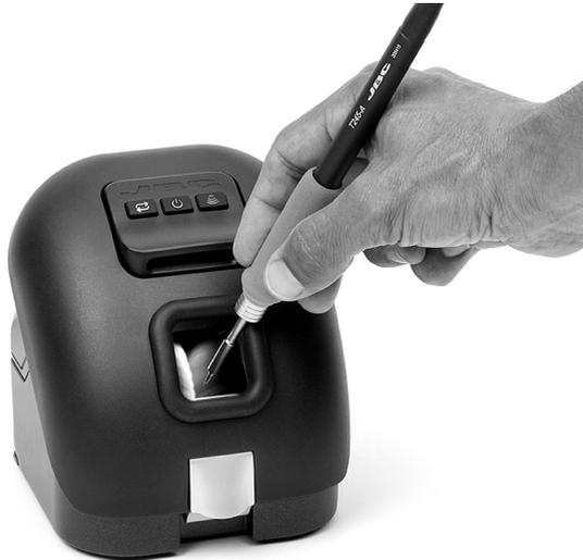
The CLMU-PA is automatically switched off if the splashguard is opened during operation.
