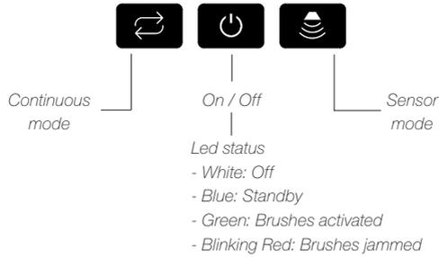
For best cleaning results, we **recommend** placing the tip between the two brushes for just 1 second. Longer exposure time would lead to dewetting of tip surface causing oxidation.
