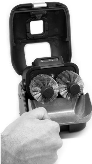
Remove the solder collection tray for disposal of solder waste.
