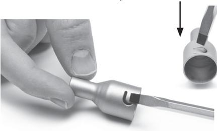
2. Insert the nozzle into the JT-TA Heater again
