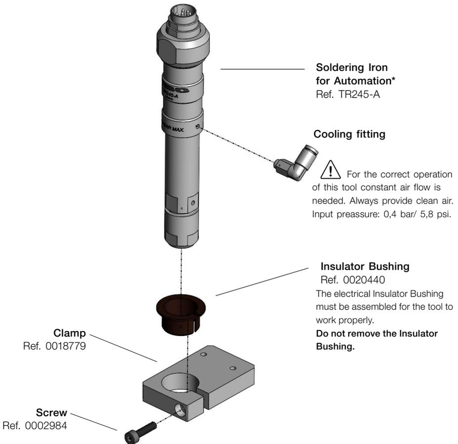
\* If the Soldering Iron is fixed in another way, it must be isolated from the fixation.
