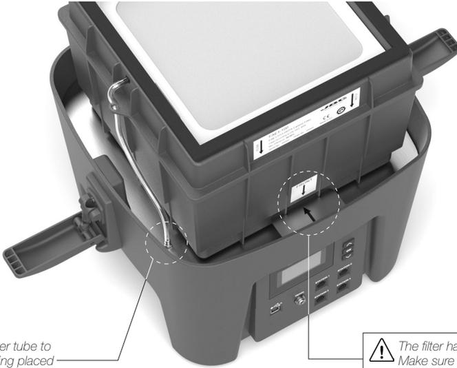
Connect the filter tube to the quick coupling placed on the metal sheet
