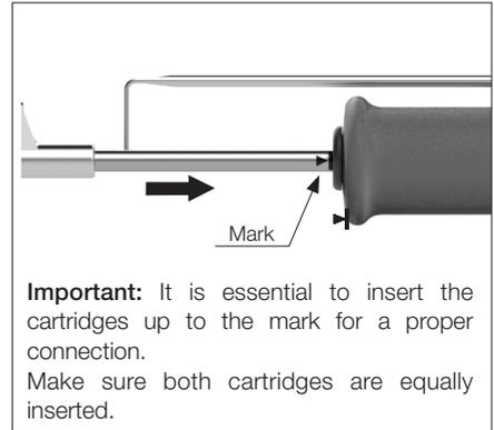
**W440 cartridges** have a proper centering to ensure a good functionality. Before tightening the screws, align the cartridges in working position using a flat pliers (Ref. PLR-195).
