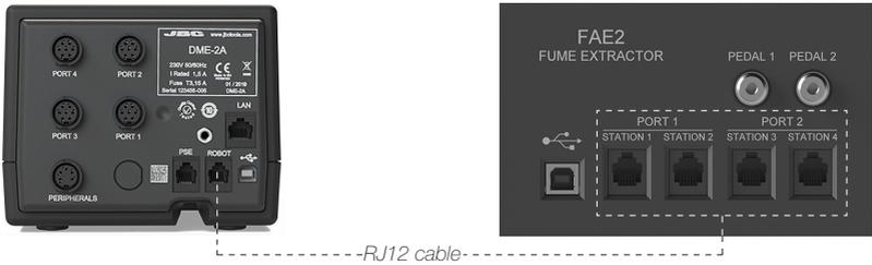
Connect up to 4 stations directly to a fume extractor through the Soldering Station Robot port. Every tool connected to a station can control the aspiration system, but previously it has to be assigned to the fume extractor through the Peripherals menu of the station. Each station detects a fume extractor as a FAE\_a.
