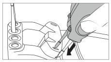
Use the grooves to insert the cartridges as far as the mark\*.
