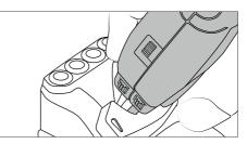
Place the tweezers on top of the new cartridge and slightly press down.
