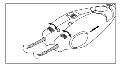
Slightly turn the wheels to align the cartridges as required.
