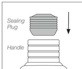
Note the Sealing Plug mounting position. The chamfered side has to be positioned towards the Handle.
