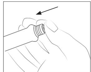
Gently push the Sealing Plug inside the handle until it is completely into the Handle. Handle and Sealing Plug edges have to be aligned.
