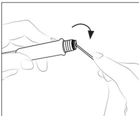
Enter a small shaft or screwdriver in order to gently lift and pull the Sealing Plug. Do not insert the tool more than 8 mm deep. Never use a cartridge to do this operation.
