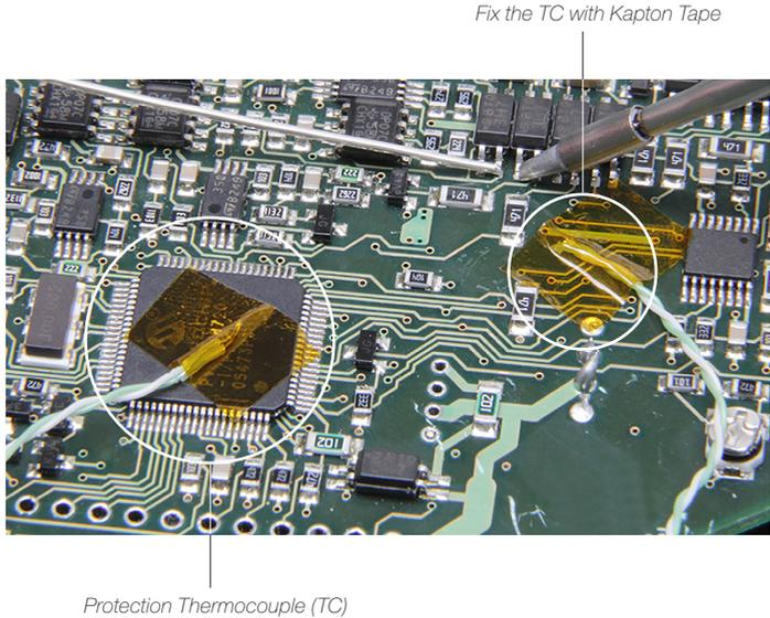
2. If there are any sensitive components, use a Thermocouple as protection.
