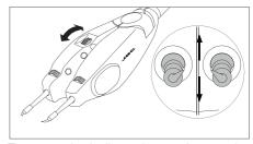
The rear wheel allows the cartritges to be equally aligned when you close the tweezers.
