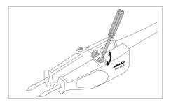
Lock the fixing screws.
