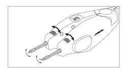
Slightly turn the wheels to align the cartridges as required.
