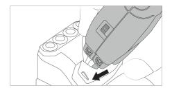
Place the tweezers on top of the new cartridge and slightly press down.
