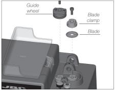
↑ \* Handle with care to avoid any cuts with the blade because it is sharp.
