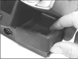
1. Insert the wiper in the cleaning place of the LC Unit Control.
