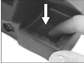
2. Press the wiper down to fix it in place.
