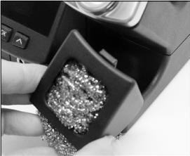
1. Put the brass wool in the dome and insert it in the cleaning place of the LC Unit Control.
