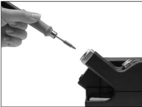
When the tool is lifted from the stand the tip will heat up to the selected temperature.
