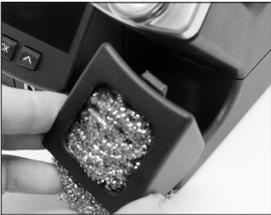
1. Put the brass wool in the dome and insert it in the cleaning place of the LC Unit Control.
