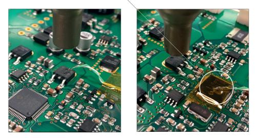
$\rm IPC^*$  does not recommend exceeding ramp-up rates over 3-4°C / sec. (5-7°F / sec) so as to reduce the risk of thermal stress on the PCB.
