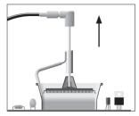
The component lifts off automatically when the solder melts.
