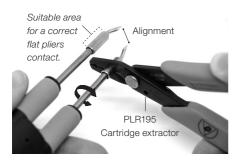
Use a flat pliers in the indicated area for a correct tip alignment.
