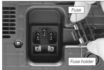
**1.** Pull off the fuse holder and remove the fuse. If necessary use a tool to lever it off.
