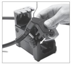
2 Insert the fume inlet duct for modular stands between the knob and the tool holder.
