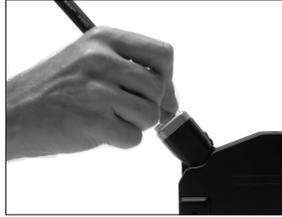
When the tool is in the stand, the temperature reduces to 180°C / 360°F (preset sleep temperature).
