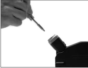
Lift tool from the stand and the tool tip will heat up to the selected temperature.
