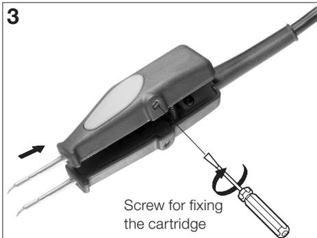
Align the tips of the two cartridges.
