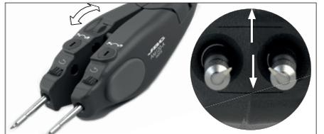
The tail wheel guarantees that the cartridges are equally aligned with vertical symmetry.
