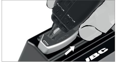
Place the cartridges in the extractor and pull the tweezers to remove them.
