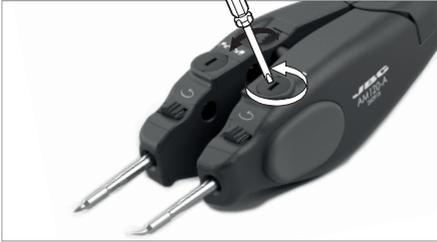
Unlock the fixing knobs.
