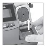
**3.** Press the wiper down to fix it in place.
