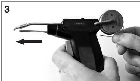
Insert the solder into its hole checking that the wire becomes straight. Pull the trigger intermittently until the solder feed system works by itself.
