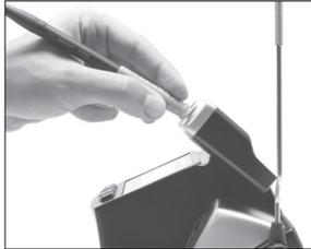
When the tool is in the stand, the temperature falls to the preset sleep temperature.
